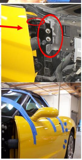
Use the fork to loosen the factory wire boot and unplug the wire harness, this will allow you to install the new VDI system. Make sure it's flat against all surfaces.
