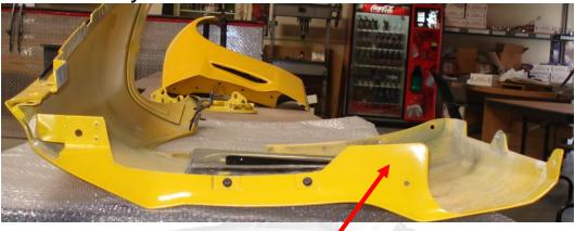
Drill new hole for support bracket. use M6x1 bolt.
