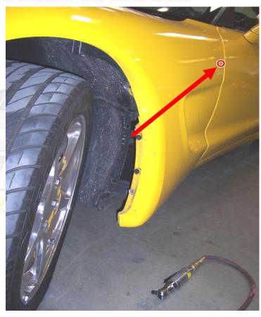
After you have removed the wheel well fasteners, reach in and remove the turn signal by disconnecting the wire harness and pushing backside clamps inward and pushing the light out.
