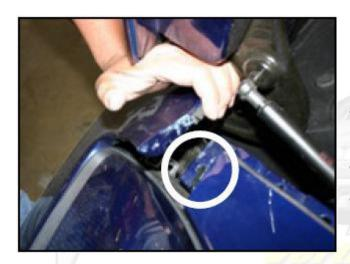
Pull upward on front bumper cover as shown and remove screw with T15 Torx wrench.
