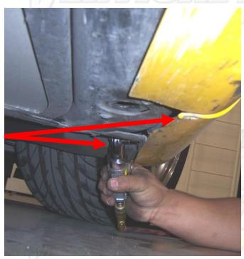
Remove (2) 7mm bolts from the bottom of the fender.
